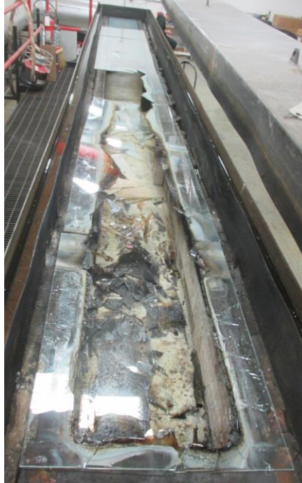
Photo No. 3 Unexposed Surface of the Test Specimen (Post-test)
